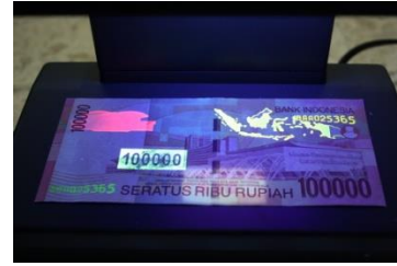
Figure 4. Ultraviolet light to detect counterfeit money [16]
