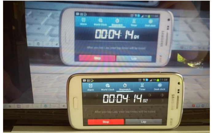
Fig. 5 a 180 ms delays between the factual and from the receiver on the monitor.
