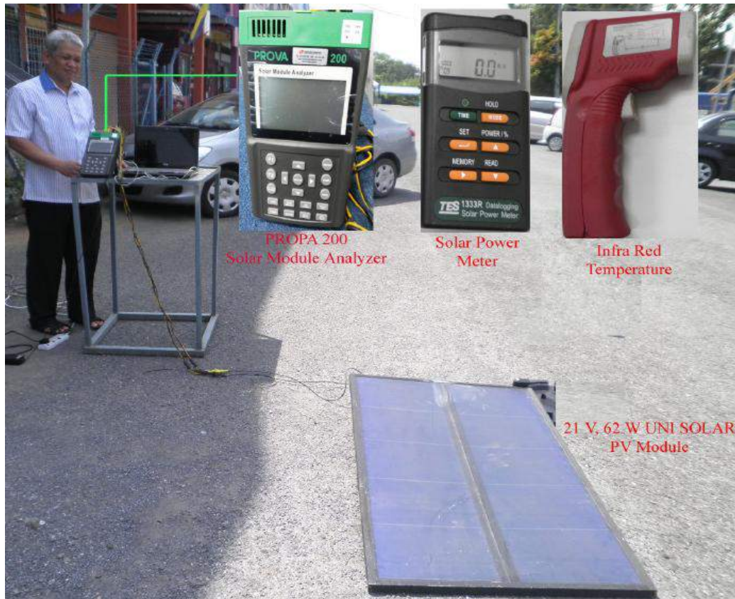
Figure 1 Measurement of PV module performance
