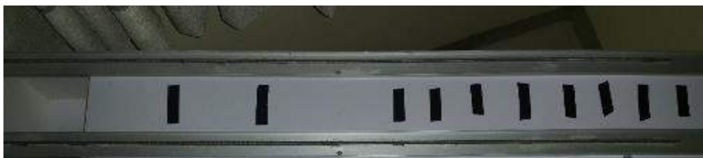
Figure 16 black line for robot position
